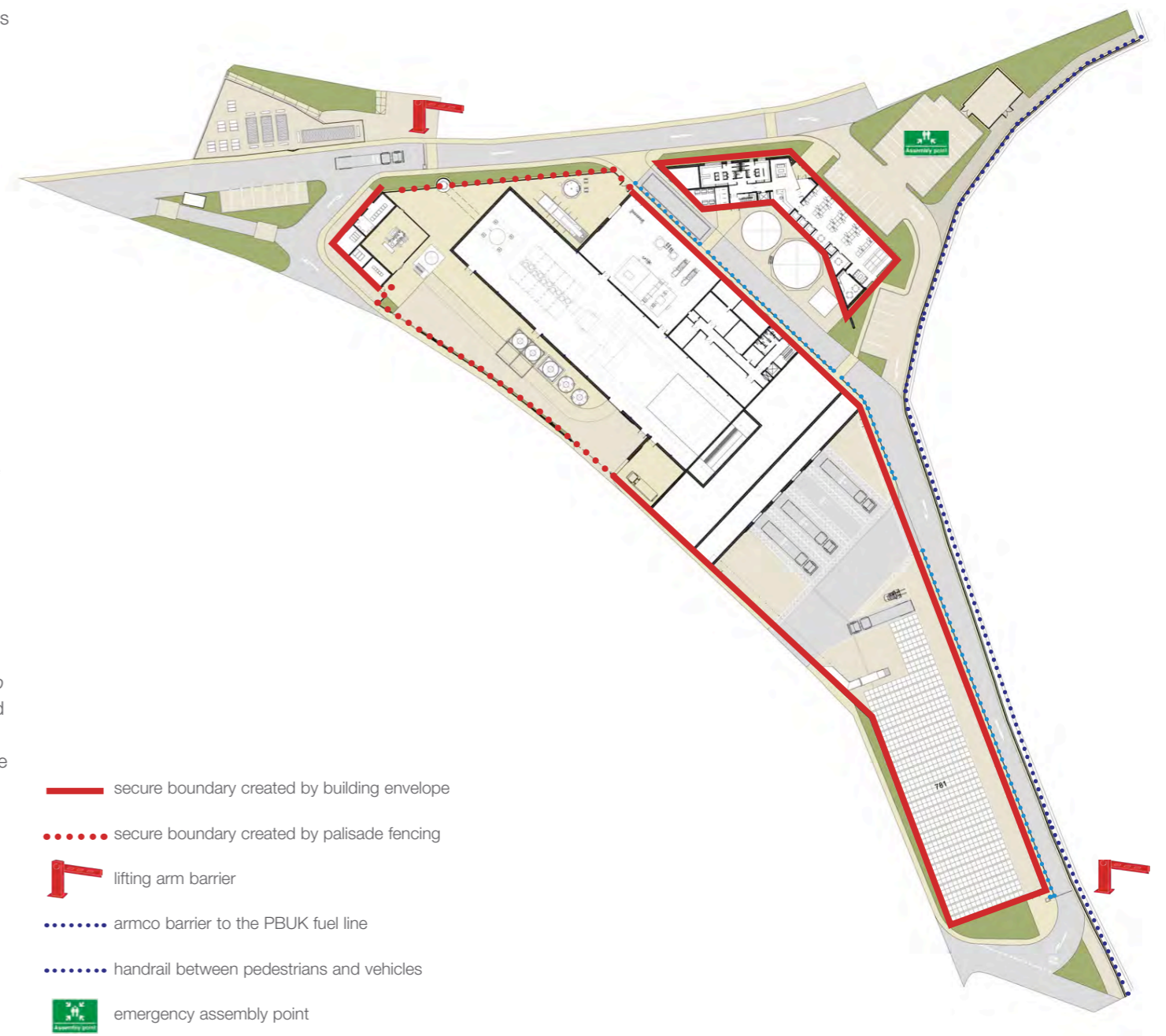
FIG 8.3 SITE SECURITY AND EMERGENCY ASSEMBLY PLAN
