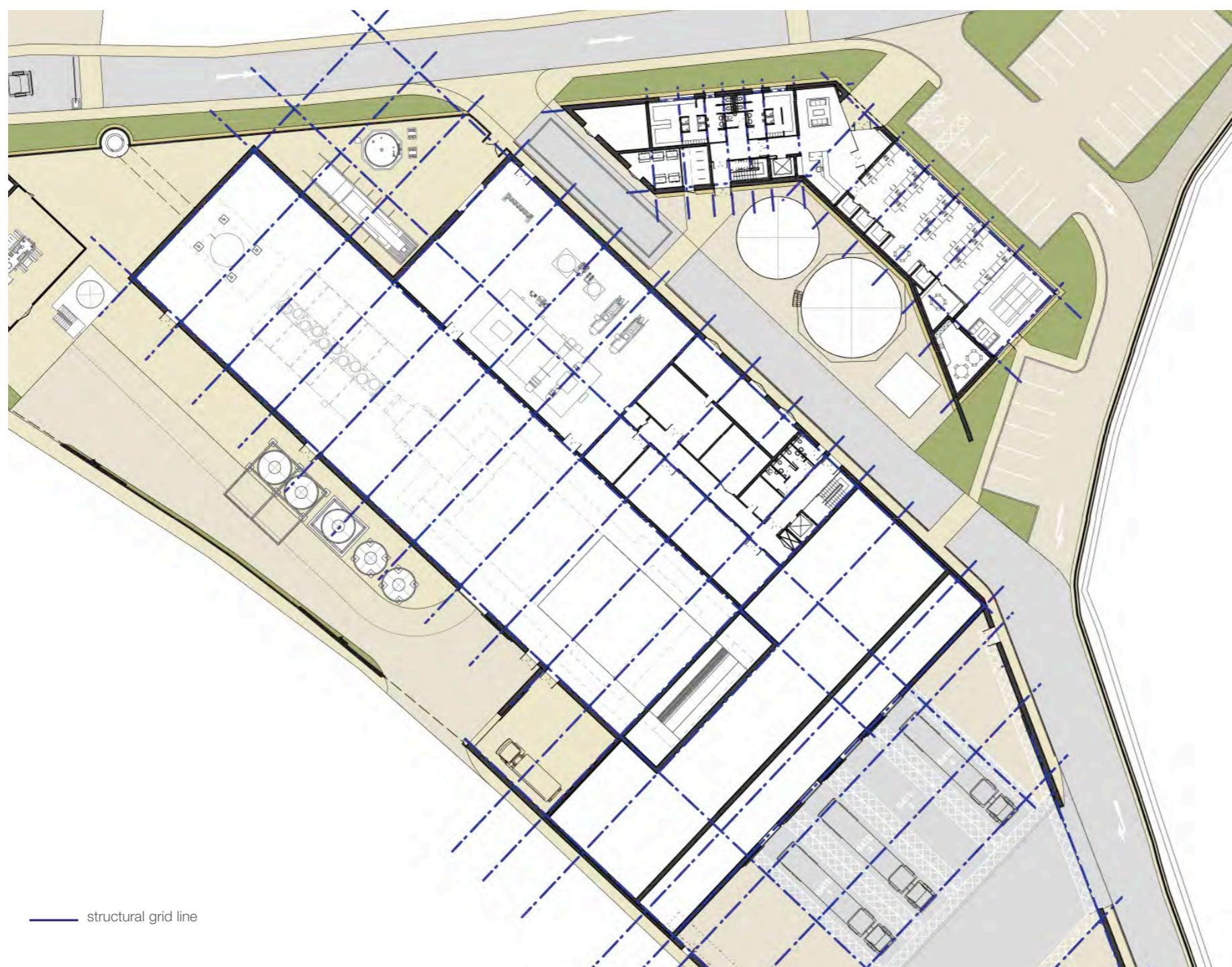
FIG 8.4 INDICATIVE STRUCTURAL GRID THROUGH PLANT AND OFFICE BUILDING
